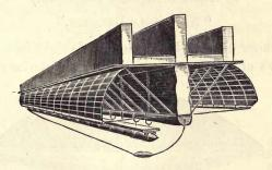
By heating an expansion-chamber the entire machine is made to displace more air than its entire weight, and thus has a lifting power. The centre of gravity is adjusted by means of a moveable weight, and the angle of the aëroplane can thus be adjusted and cause the ascending or descending force to propel the machine ahead.
